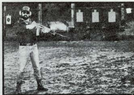
Author fires the Galil into the same mud that the weapon was dropped into repeatedly. Even after complete mud bath the weapon functioned flawlessly.
