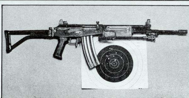
After 800 rounds of ammo, no cleaning, and with test gun still showing signs of dried mud on exterior, the Galil shot excellent 10 shot groups at 100 yards.
