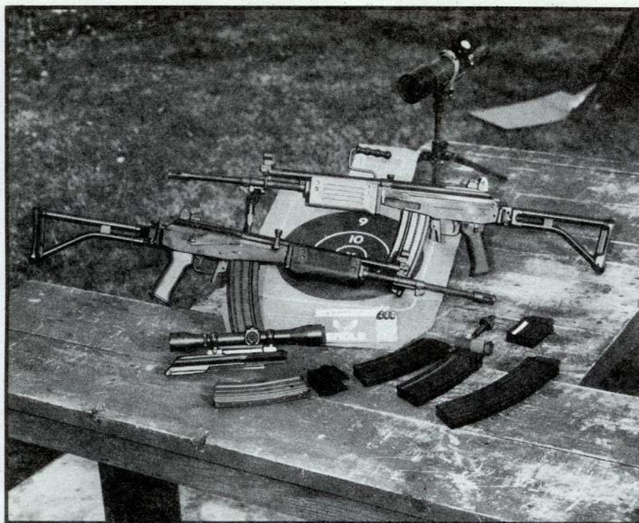
Magnum Research, Inc. .223 AR (bottom) and ARM (top) with accessories. Note scoped top cover, M-16 magazine adapter as well as various magazines. Center magazine is for blanks, and blank adapter is atop.
