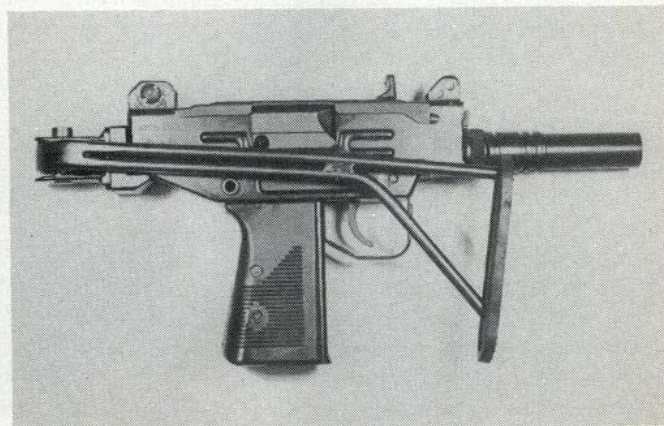
The folding stock makes a handy front grip. Muzzle extension was added to move the muzzle blast away from forward arm.
