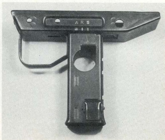
The pistol trigger housing is very similar to that of the carbine and can have the selector markings added in the same way (see Uzi carbine article on page 59).
