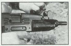
Like the Uzi carbine, shown here, the Uzi pistol is cocked by pulling back on the charging handle while holding in the grip safety.
