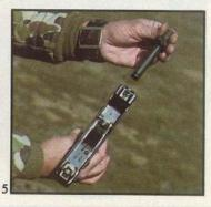
Fieldstripping the pistol is a simple task. First remove the magazine and cycle the action, making sure the Uzi is empty. Release the catch holding the breechbolt cover and remove it (photos 1 & 2). Pull the breechbolt rearward about one inch and lift up on the front of it (3). Continue lifting up at the front and the breechbolt will then clear the frame (4). Holding in the catch securing the barrel nut, unscrew the nut and remove barrel.
