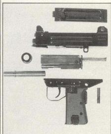
When fieldstripped for cleaning the pistol breaks down into three basic units; frame, breechblock and barrel.
