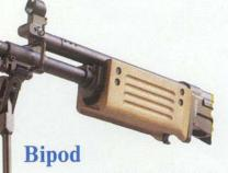
The Galil Model ARM is one of very few assault rifles with a built-in bipod. The Galil's bipod is strong, won't break or deform when slammed on the ground and contains a wire cutter.
