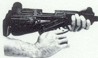
Barrel The barrel is removed by pressing the catch beneath the front sight and unscrewing the barrel-retaining nut from the receiver.
