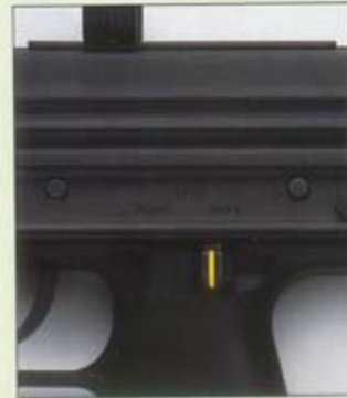
A three-position safety/selector lever allows semiautomatic or full automatic firing.
